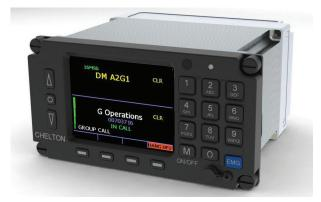
from the displays is LED white. Maximum NVIS radiance is within the MIL-STD-3009 published limits for 'multi-colour' electro-optical displays.
