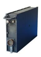
The connector interfaces are accessible from the front faceplate of the unit. The unit is designed to be rack mounted in a short tray.
