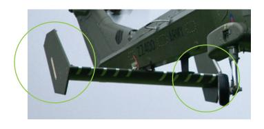
The V/UHF element is configured as a broadband top-loaded monopole. The lower portion of the end plate is metallised to act as a counterpoise for the element and to provide a source of grounding in order to optimize the RF performance commensurate with meeting the lightning specification. The element is fed via a susceptance compensation network to maximize VHF gain. Frequency dependent resistive loading ensures compliance with the return loss limits.
